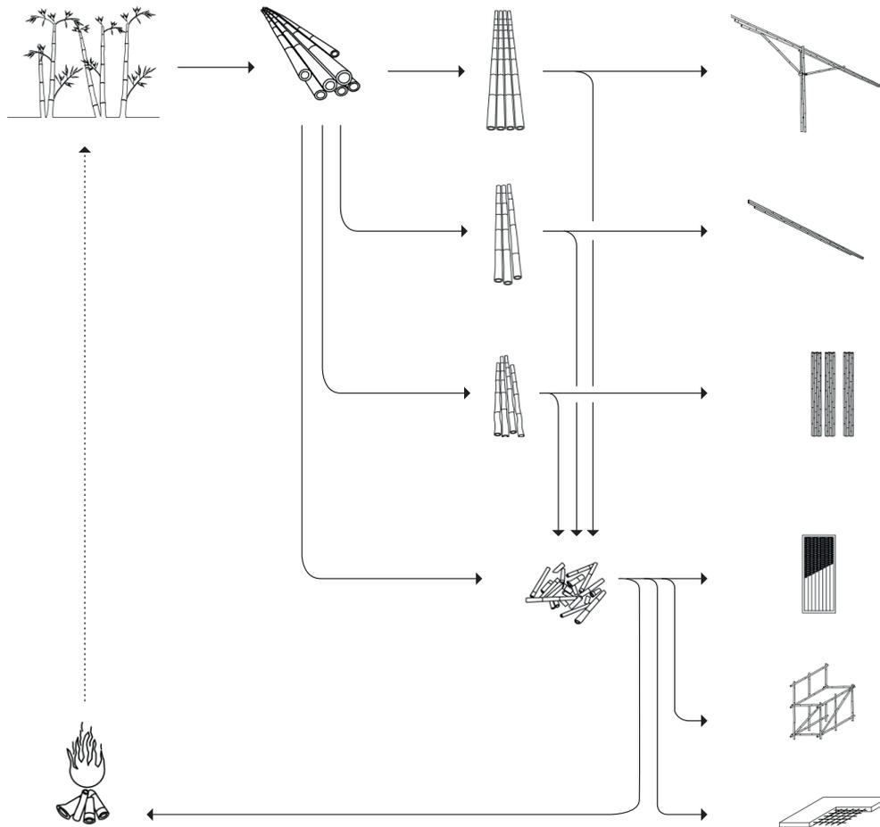
*fig. 10 cascade sorting system for different types of construction elements*
