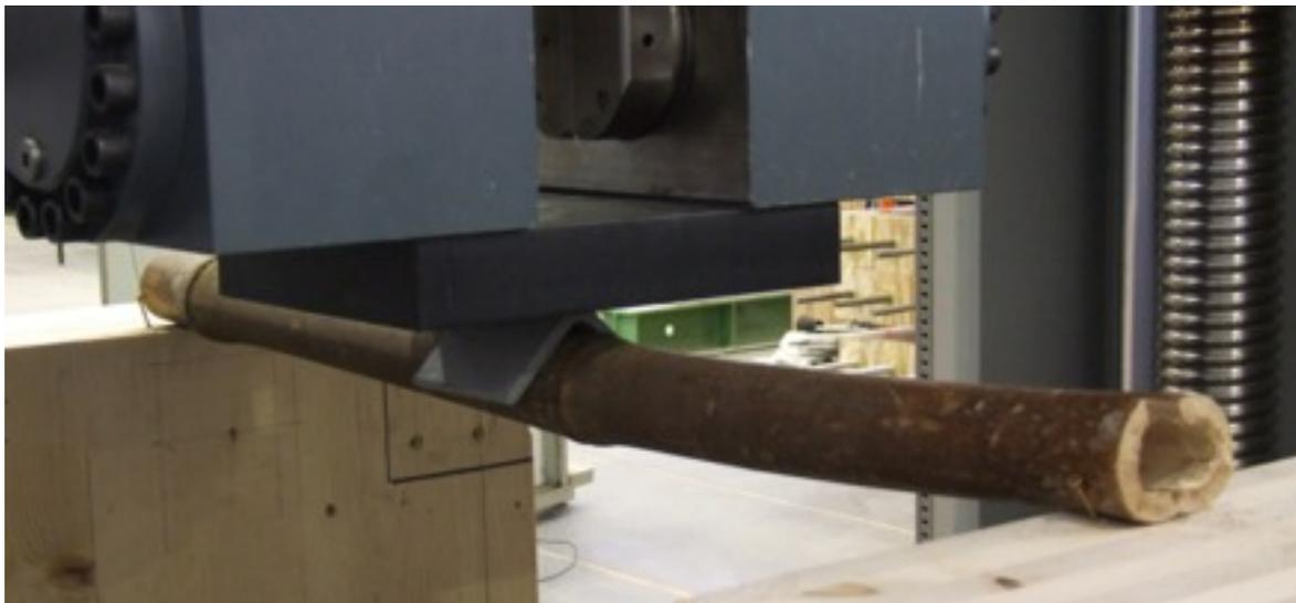
fig. 8 Material testing of samples of Kenyan *Yushania Alpina* at the TUM: Cracking cane by punktual strain at the support
