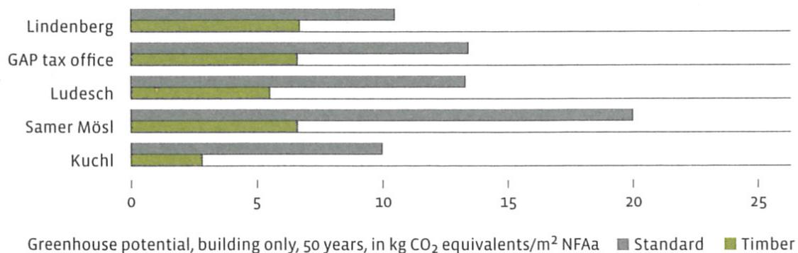
fig. 5 Greenhouse potential of timber construction compared to conventional construction at the example of five building ensembles in Germany and Austria
